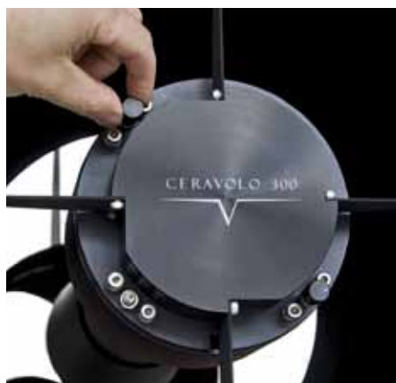
Collimating the scope is easy. Just turn one of the two knobs that control the orthogonal motion of the secondary mirror.
