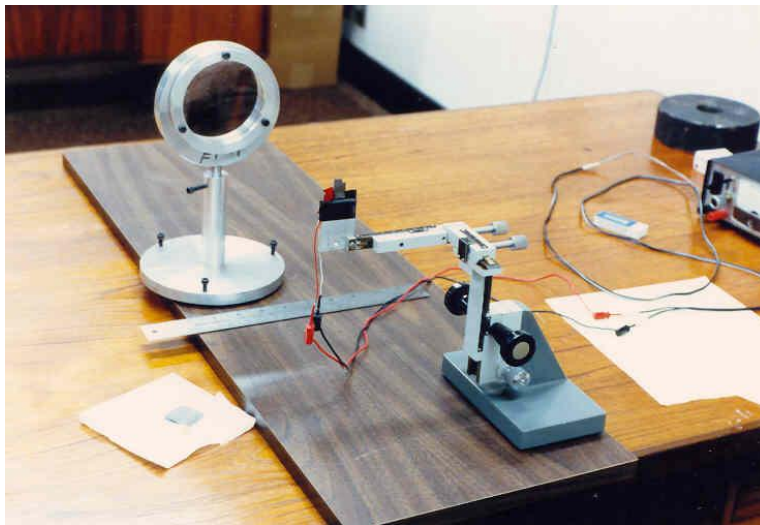
This set-up of the author's Ross null test was used for many years to produce a variety of mirrors
