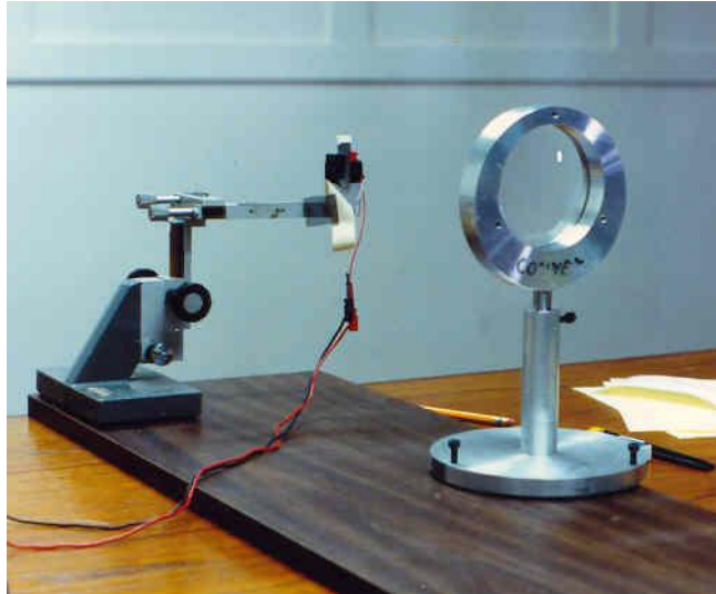
The author's 3.5" Ross null lens in a simple holder. Note the 1" square Ronchi grating dangling from a piece of tape.
